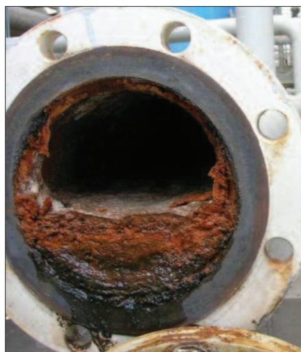
*Scale, biofilm, and corrosion deposits within pipework.*
