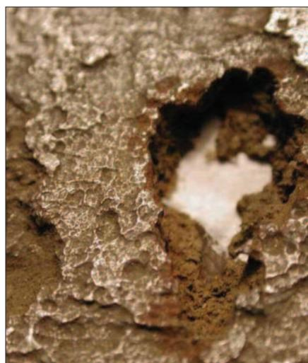
*Corrosion pit and subsequent leaking pipework.*
